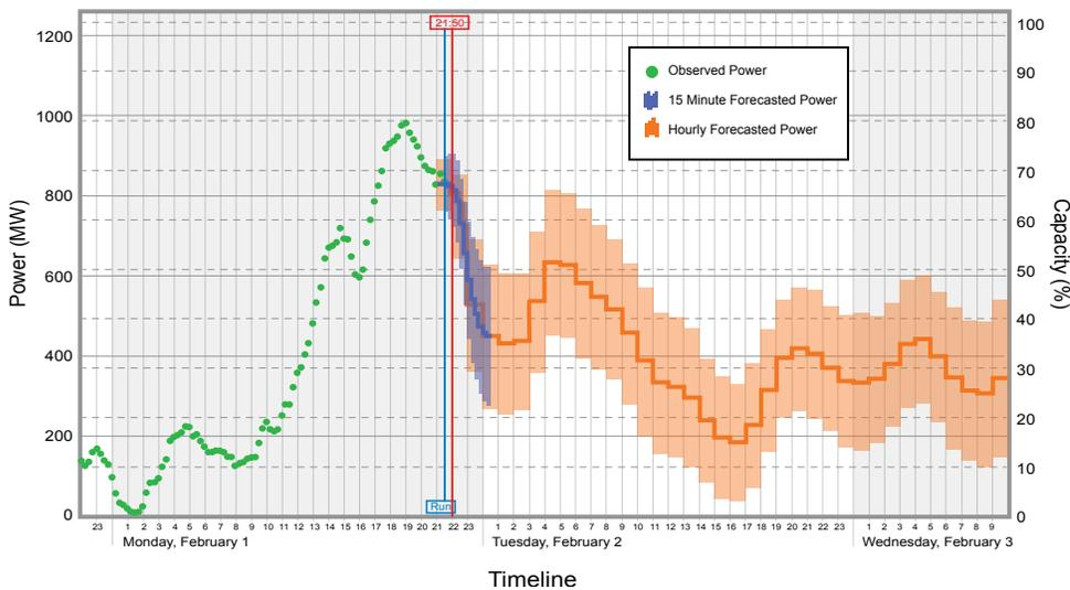
Many power systems with relatively high shares of wind power have integrated wind forecasting into system operations. This graphic, based on sample wind forecasting output for Xcel Energy (a utility in the United States), shows a wind power forecast over a 36-hour horizon, including actual power generation (green dots) up to the initial forecast point, the predicted wind power (solid line), and the typical forecast error from the preceding seven days (shaded area) [1].
