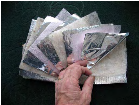
Thin reflective foils separated by thin air layers have a very high insulation value because they block the infrared heat radiation.
