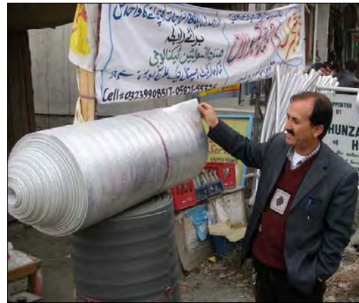
Thin reflective foils separated by thin air layers have a very high insulation value because they block the infrared heat radiation.
