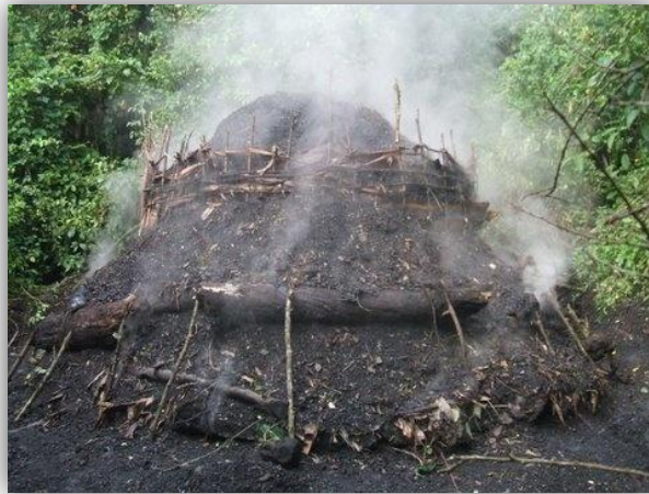
Figure 7 - Typical Traditional Earth Mound Kiln used in the region (Virunga NP, 2008)
