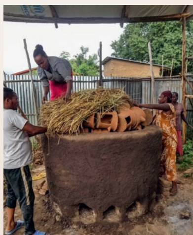
Bottom from left to right: Scaling clay stove production with simple tools; Kiln with clay stoves before firing; Kiln loaded with clay stoves during closing and sealing preparation; Transportation of clay stoves - Improvement is needed to reduce breakage rate.
