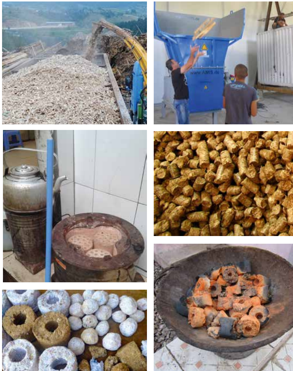
Figure 2.4 Downsizing in a chipper (top left) and grinder (top right). Densified solid biomass fuels examples.
