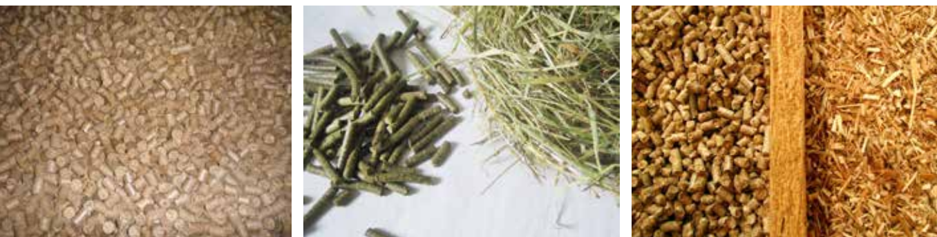
Figure 2.10 Pellets made from tobacco stalks (left), hay (center) and Miscanthus straw (right).
