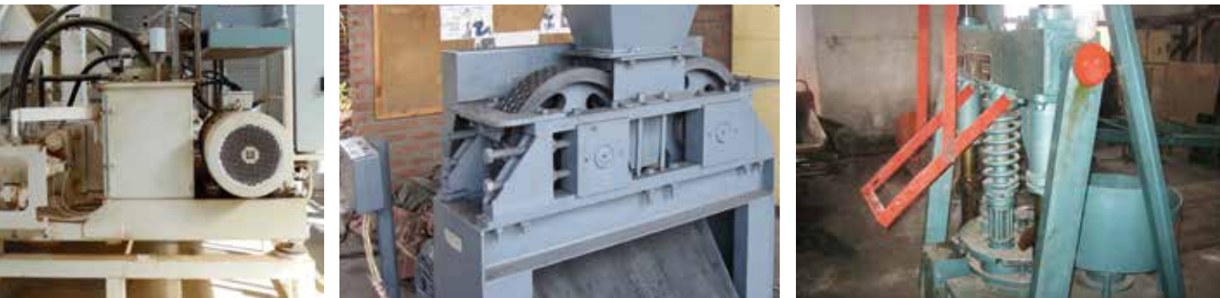
Figure 2.7 Three different types of briquette presses. RUF press for wooden briquettes (left), roller press for carbonised pillow-shaped briquettes (center) and press for carbonised honeycomb briquettes (right).
