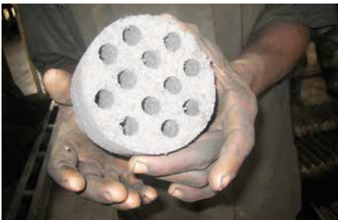
Figure 2.6 Two charcoal briquettes with inherent design that supports low emission and complete combustion.
