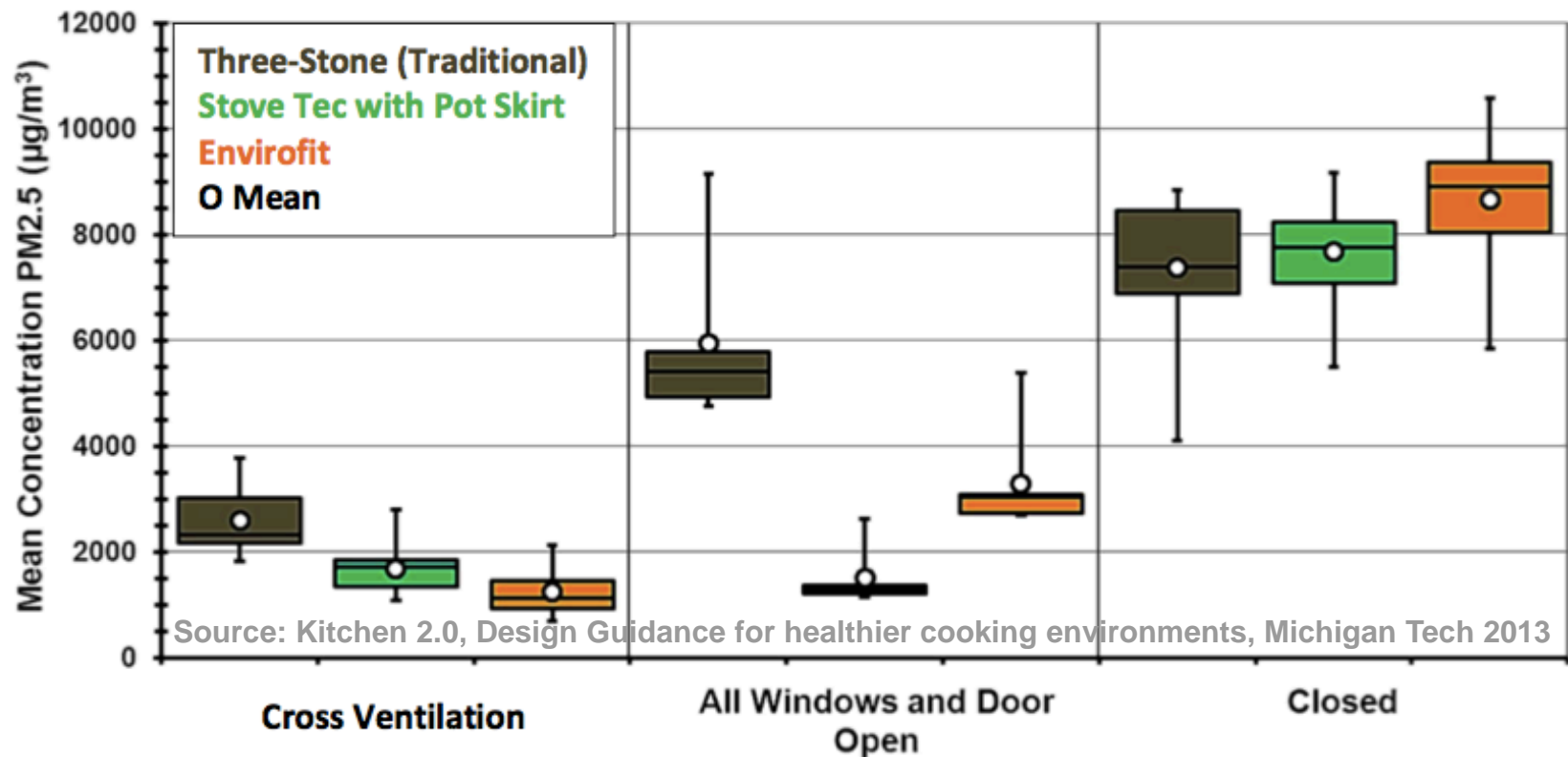
Figure 4: Depicts UCB monitors' mean averages (n=3) for three stoves under three ventilation variations at standing (60cm) and sitting (39cm) heights (steel roof only) . Averages calculated during first 45 min of trials.
