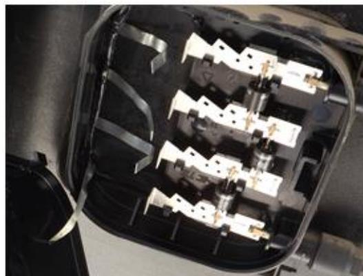
FIGURE 41: SOUDURE INEXISTANTE DANS BOITE DE JONCTION. MODULE NON OPERATIONNEL ET RISQUE D'INCENDIE REEL
