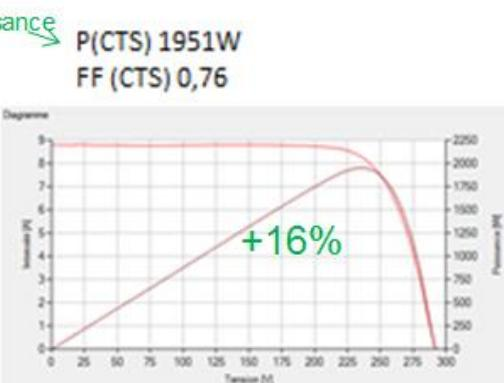
FIGURE 29: EFFETS DU NETTOYAGE SUR LA COURBE I(V)
