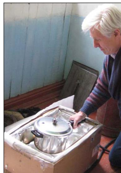
Heat-retention cookers are commonly made from insulation materials such as Expanded Polystyrene, EPS ( $\lambda=0.04$  W/m.K), loose wool ( $\lambda=0.05$  W/m.K), straw ( $\lambda=0.08$  W/m.K) or even less insulating materials. However, the highly reflective metalized foils are far more effective and require less space.
