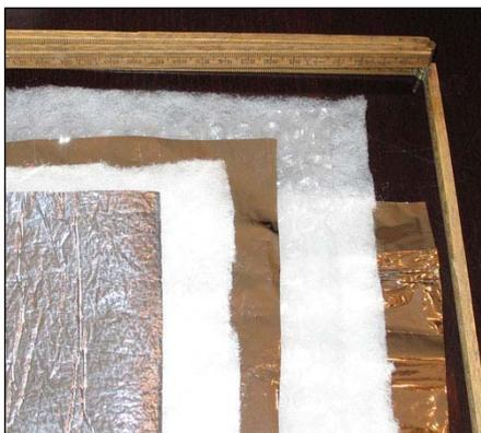
This metalized insulation foil is commonly used for pipe insulation, under laminate floors and for house insulation. It is becoming widely available.
