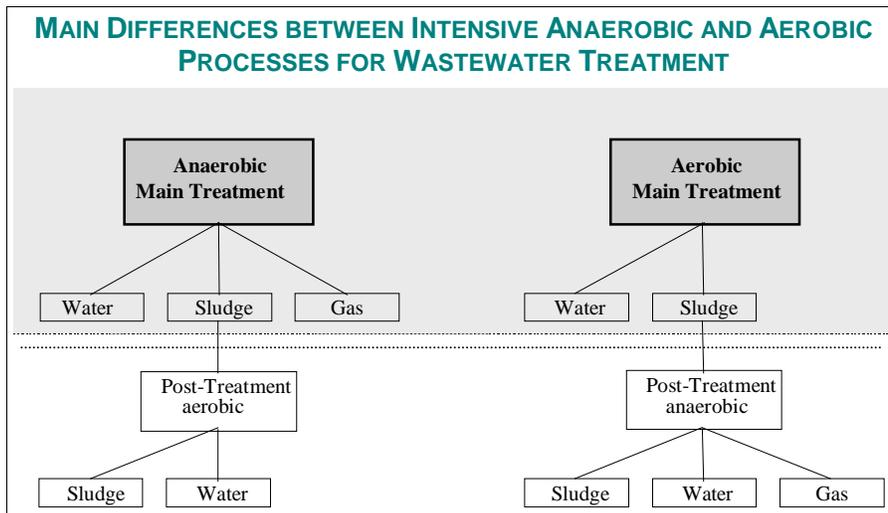
**Fig. 2: Difference between anaerobic and aerobic processes**
