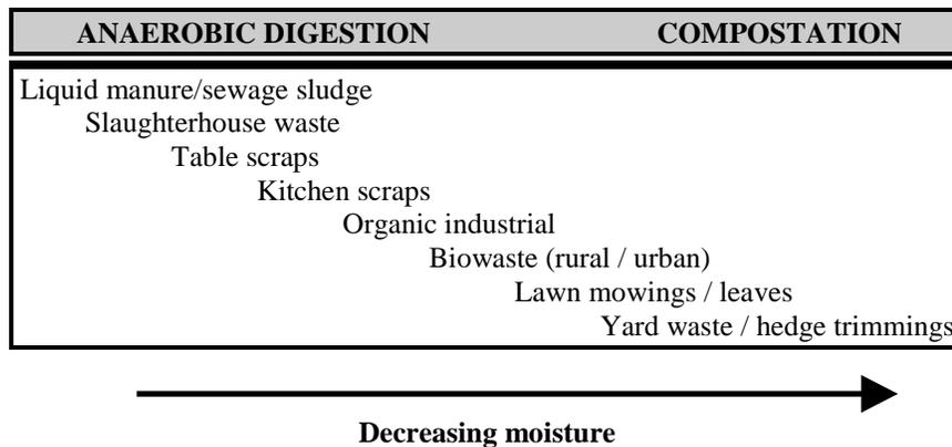
Fig. 4: Suitability of organic waste for anaerobic digestion or compostation
