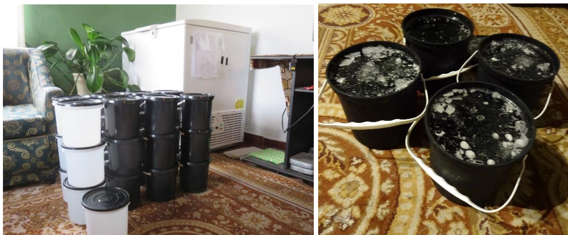
Fig. 7: 25 ice tins in total for the CPT-Kit for producing 2 kg-ice-buckets
