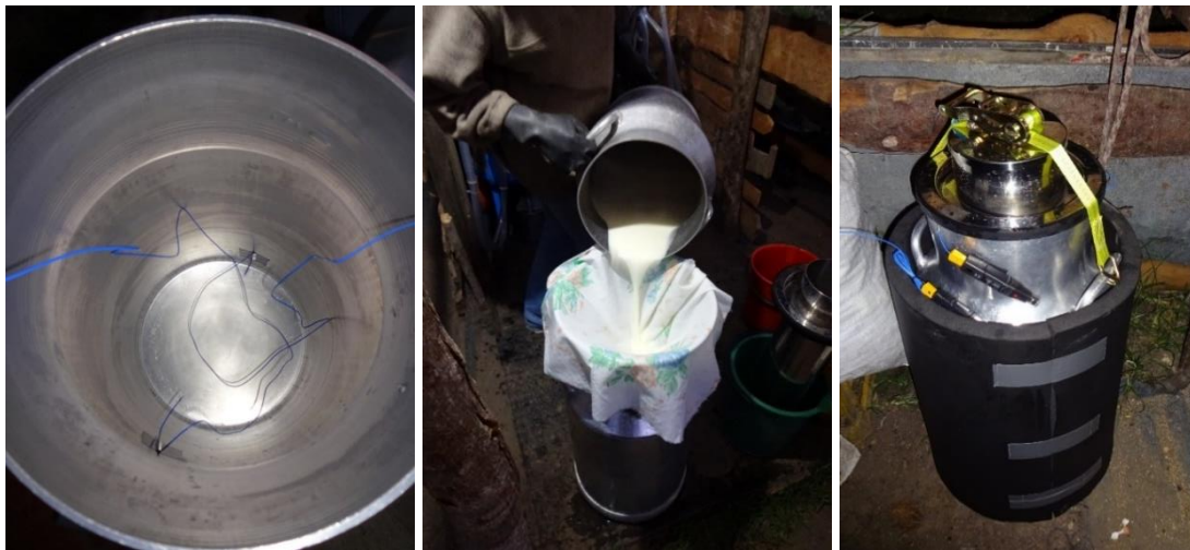
Fig. 8: Position of the thermocouples (left), sieving of the milk (middle) and measurement during overnight storage (right)
