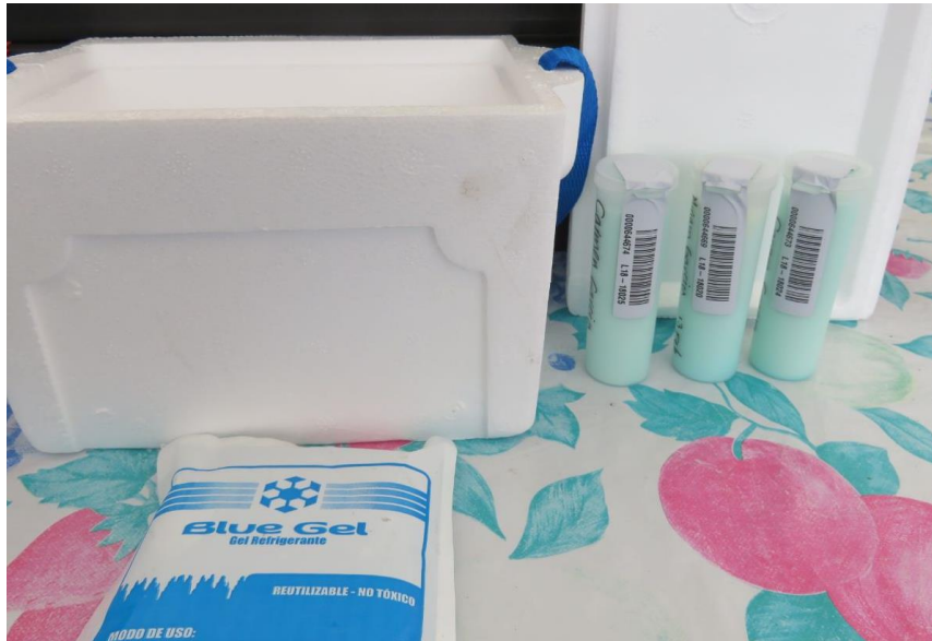
Fig. 13: Milk sample storage with the tubes, the polystyrene insulated box and refrigeration gel for keeping the samples below 4°C.
