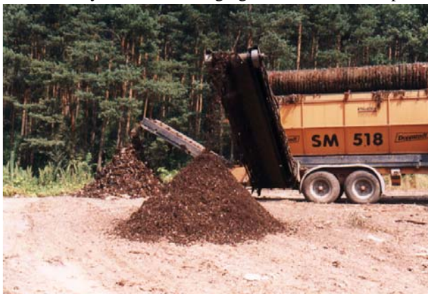
FIGURE 2 Segregation of methane oxidation material
