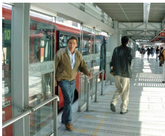
Fig. 12 TransMilenio has the look and feel of a rail system, but with the operational costs and other advantages of buses. Bus stations and bus doors are elevated, allowing quick boarding and alighting.
