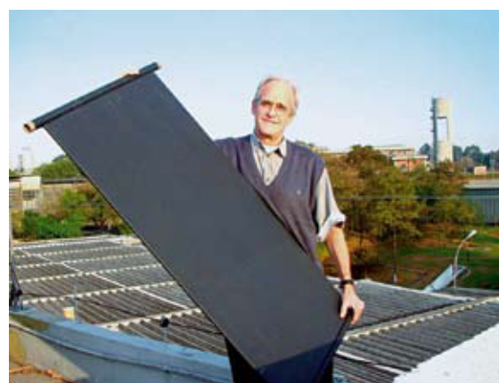
Photo: Sociedade do Sol – Presenting the black painted PVC collector.
