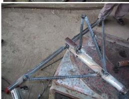
3. Weld two 6 cm long pieces of a pipe with a diameter of 2.5 cm to the other end. Place 6" screws into the holes of the 6 cm long pieces of pipe. To strengthen the rig further, weld concrete reinforcement iron to the T-form as shown in the pictures below.
