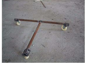
On the T-form, find a spot with equal distance to every roller and weld a 24 pipe with a diameter of 2.5 cm. Weld a ring of 14" steel rod at one third height of this pipe and weld a length of 14" steel rod to one roller each.
