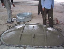
14. Cover the cement with plastic foil and let dry for two days. Remove the plastic foil on the second day and let the cement dry for an additional 3-4 days. During this time, pour water over it several times. After 3-4 days the solar cooker is taken from the form and turned upside down. The solar cooker has to dry for an additional three weeks.
