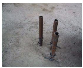
3. Put the piece of pipe in the middle of the flat iron ring and fill it with cement. After several hours, remove the flat iron ring and let the stand dry.
