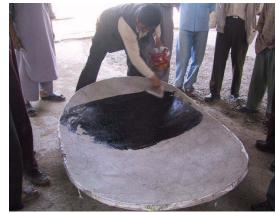
Cut the glass into long pieces and cut those pieces into small squares with a length and width of 1.5 cm each. Break one square at a time from the glass to glue it to the solar cooker.
