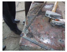
9. Weld the ring to the bent piece of iron.
