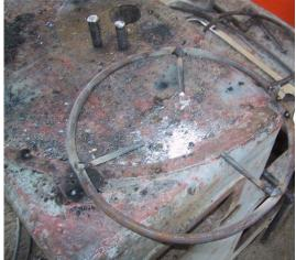
8. Cut a piece of 20" concrete reinforcement iron to a length of 1.05 m, make a shallow cut at a height of 20 cm, bend the piece of iron at 90 degrees and weld together.
