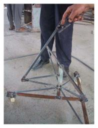
7. The last step in the production of the rig is the construction of a pot holder. The pot holder is made of 20" concrete reinforcement iron, 10" iron rod and 8" iron rod. First cut a piece of 10" iron rod to a length of 80 cm and bend it into a ring. Weld three pieces of 8" iron rod with a length of 5 cm each into the ring.
