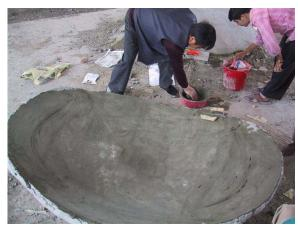
After the form has dried the master form can be used for the production of the transportable form.
