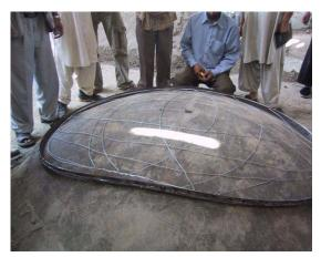
8. Riddle the coarse-grained sand and mix it with cement in a 2:1 ration. (One sack of cement should last for two solar cookers.) Put the flat iron ring and the iron wire mesh onto the newsprint.
