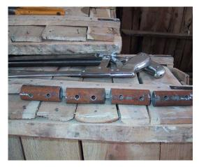
2. Weld 30cm of a pipe with a diameter of 3.3 cm, 65cm of pipe with a diameter of 2 cm (or 20" concrete reinforcement iron), and one 6 cm piece of pipe with a diameter of 2.5 cm as shown in the picture.
