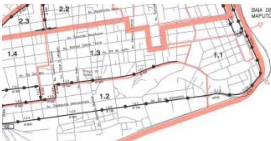
Preliminary design of the main components of the proposed sewerage in the centre of Maputo
