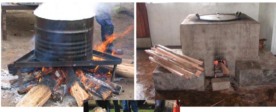
170 kg on the open fire 14 kg with the new rocket stove
