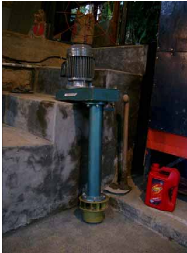
Figure 4-16: Indonesian manufactured small, unregulated Francis turbine, coupled to an IMAG (ca. 0.6kW)
