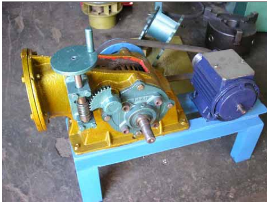
Figure 4-13: Small, fully operational cross-flow turbine (ca. 1kW), coupled to a small IMAG. Turbine manufactured locally in Indonesia.
