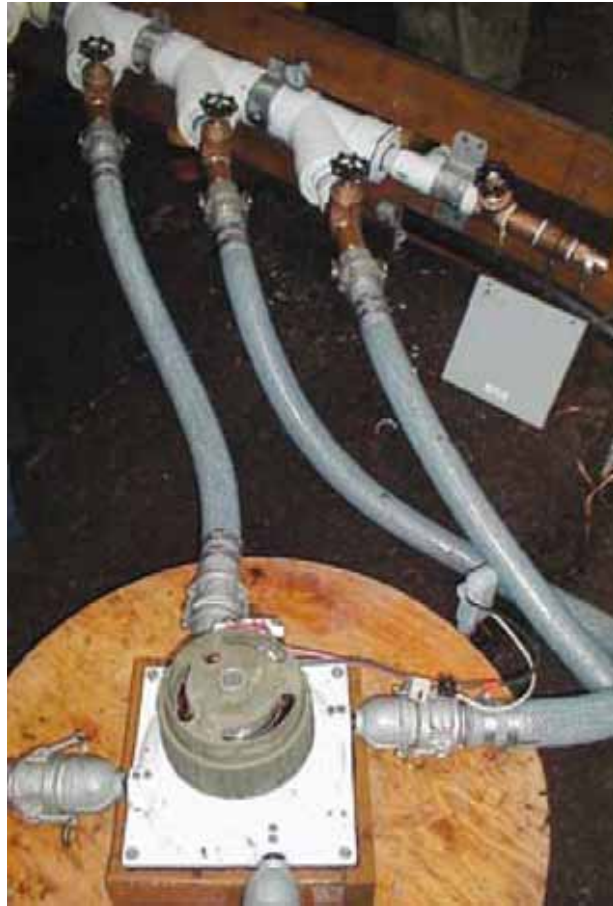
Figure 4-6: Small, self-made Pelton turbine with 4 jets, driving a small permanent magnet alternator. Source: Home Power 103 / October & November 2004 / Intro to Hydropower [p.18]
