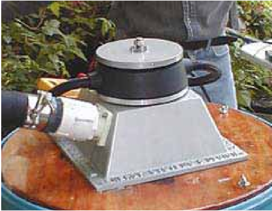
Figure 4-9: A Canadian-made Energy Systems and Design turbine uses a permanent magnet alternator and a Turgo runner. Source: Home Power 103 / October & November 2004 / Intro to Hydropower p.19
