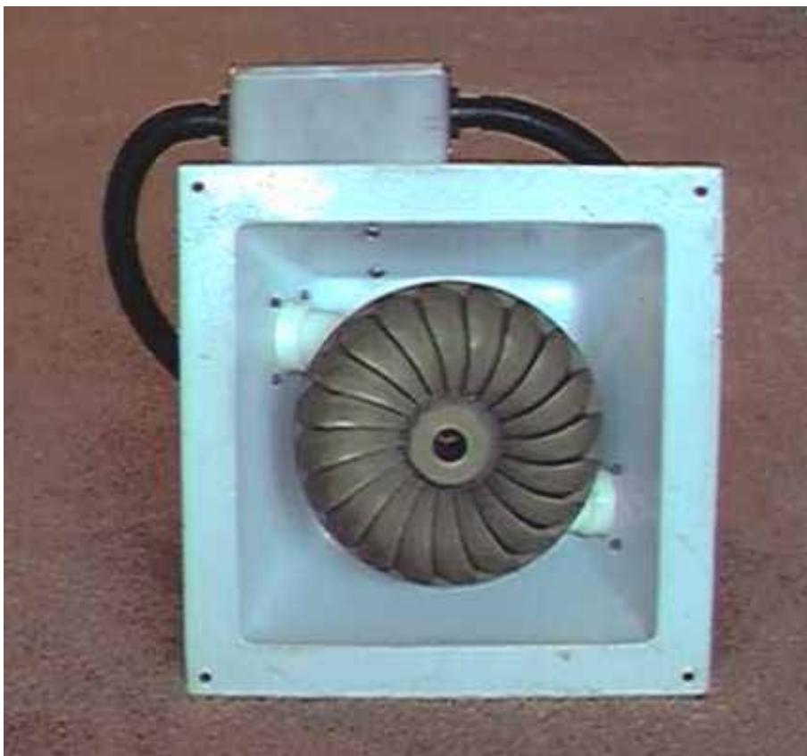
Figure 4-10: Bottom View of a Turgo Pico Turbine. Runner is made of bronze; the housing is made of cast aluminium. Source: www.hydropower.ca
