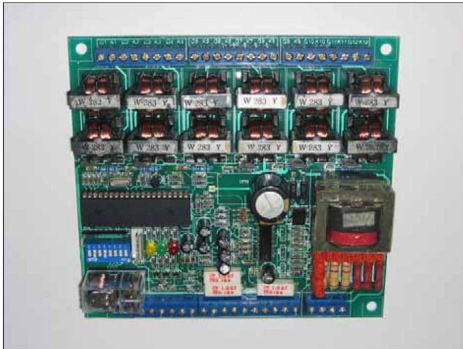
Figure 4-33: ELC for small MHP schemes (several hundred Watt), locally manufactured in Indonesia. Source: PT. Heksa Indonesia.
