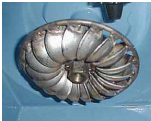
Figure 4-8: Small Turgo wheel like used in the Australian manufactured "Platypus" turbine. Source: Home Power 103 / October & November 2004 / "Intro to Hydropower" p.18
