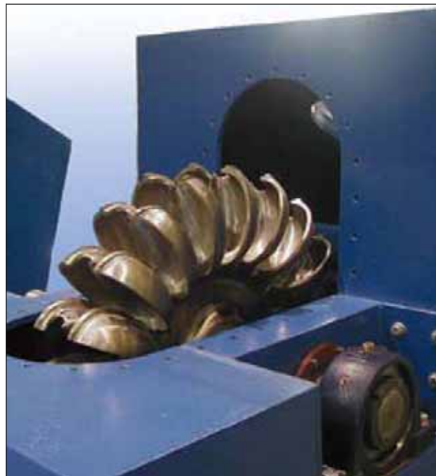
Figure 4-5: Pelton wheel with a diameter of about 60 cm Source: Home Power 103 / October & November 2004 / "Intro to Hydropower" p.18
