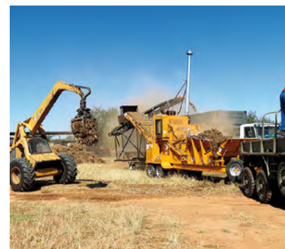
Process of feeding biomass into the chipper/grinder (WoodCo)
