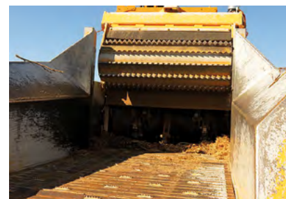
Large grinder infeed channel (Courtesy TriCycle, Langebaan)
