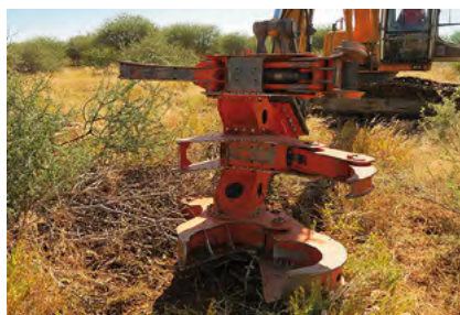
Hydraulic grab and cutter fitted to an excavator (Courtesy WoodCo, Okahandja)
