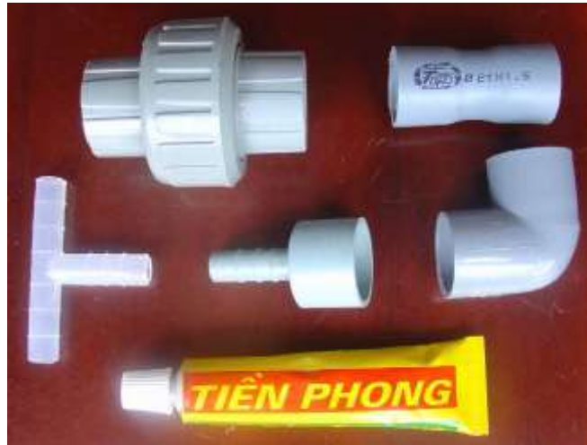
Figure 2.37. Joints: pipe connection, tee-type joint, glue
