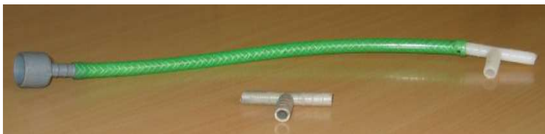
Figure 2.36. Soft pipeline connecting main gas pipeline to pressure gauge, burner and biogas lamp.
