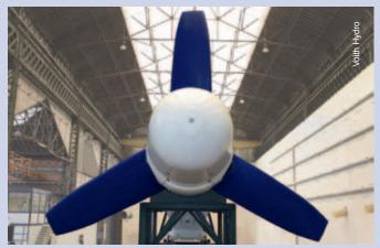
Cherbourg, France: A megawatt tidal current turbine after final assembly. The turbine was developed specifically for use in rough offshore conditions.
