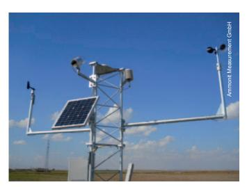
Solar measurement for site analysis: The solar radiation at the planned site of the solar park must be evaluated in order to get effective, profitable solar projects off the ground.
