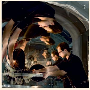
Linear solar simulator for receiver tests in the QUARZ laboratory in Cologne, Germany.
