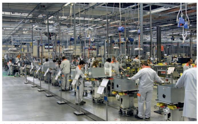
View of a production line for wall-mounted gas boilers at the company's head quarters in Allendorf (Eder), Federal Republic of Germany.
