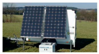
The energy-self-sufficient LiDAR measuring system of BBB Umwelttechnik.
