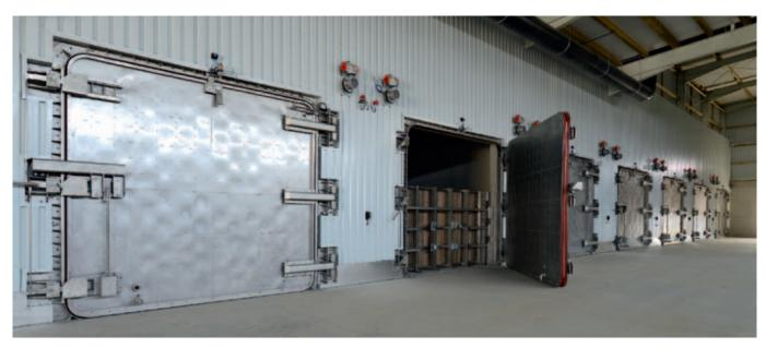
Gate system with substrate barrier in the mixing building.
