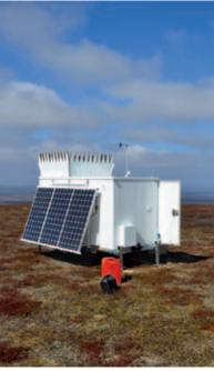
Ammonit remote sensing systems (SODAR + LIDAR).
