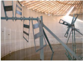
Interior view of a COCCUS fermenter with Remex paddle agitators.
