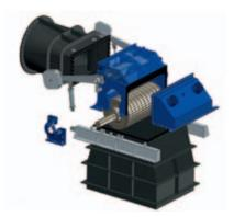
Exploded drawing of the original OSSBERGER® cross-flow turbine.
