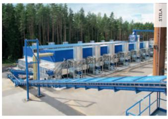
Graanul, Latvia: This low-temperature conveyor drier dries chips with an initial moisture level of 50 per cent to a residual content of roughly 10 per cent with the aid of low-calorific heat (drying temperature  $60-100\,^{\circ}$ C). Then the chips are processed into pellets. The heat used for the drying process comes from a cogeneration unit.
