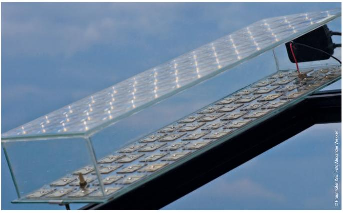
FLATCON® concentrator module with an efficiency of 36.7 per cent.
