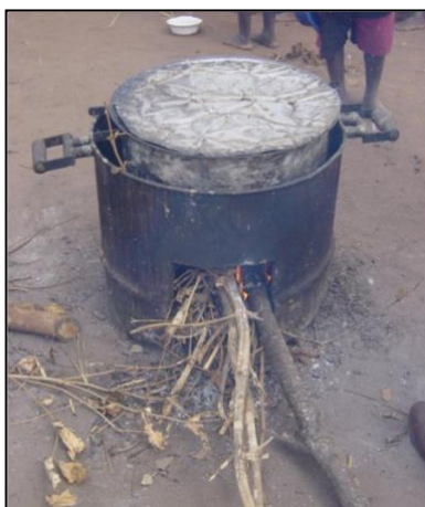
Figure 9: A low-tech portable woodstove used in a primary day school feeding programme, Mchinje District
