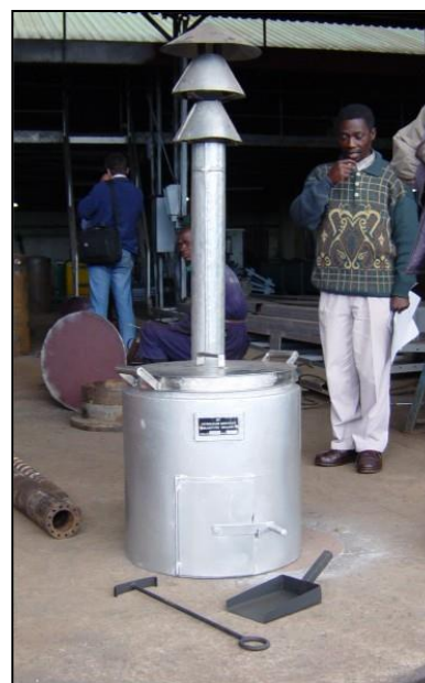
Figure 8: A 50 litre steel stove of the Bellerive 'Hoteli 50' design at Petroleum Services Ltd., Blantyre
