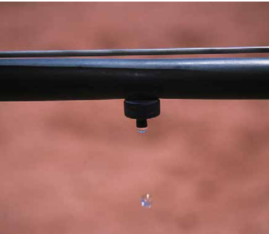
Figure 1.13: Drip irrigation pipes with mounted (on-line) emitter Source: Jeff Vanuga/ USDA Natural Resources Conservation Service / Public Domain, 2011
