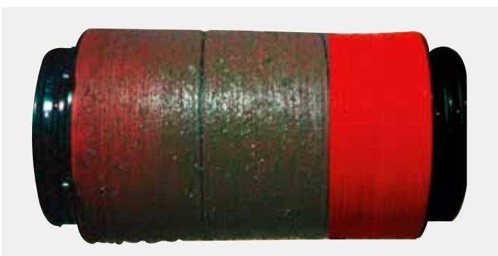
Figure 2.42: Disc filter before and after manual cleaning Source: GIZ / Reinhold Schmidt, 2015
