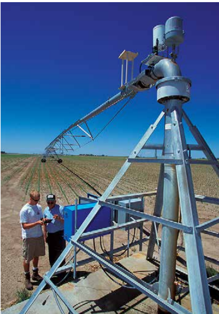
Figure 1.6: Example of a centre pivot sprinkler irrigation system Source: Scott Bauer, USDA Agricultural Research Service, 2004
