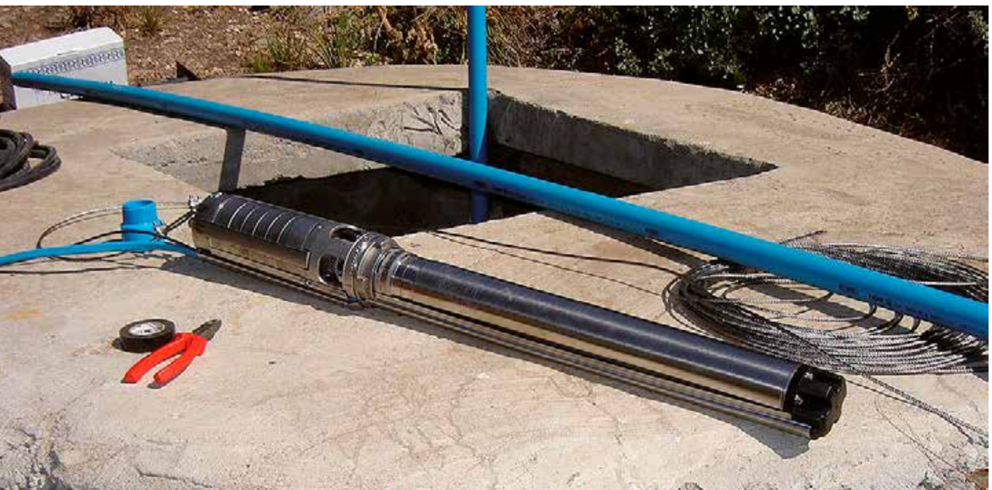
Figure 2.12: Submersible multistage centrifugal pump with integrated inverter
