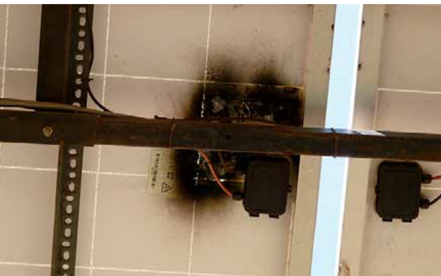
Figure 5.11: Hot spot effect encountered on no-name panel (Chinese origin) in Kenya
