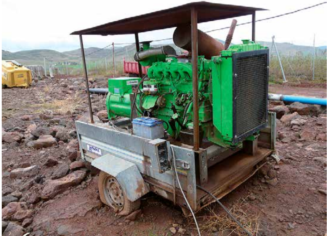
Figure 3.3: Example of an average, maintenance-demanding diesel pump set
