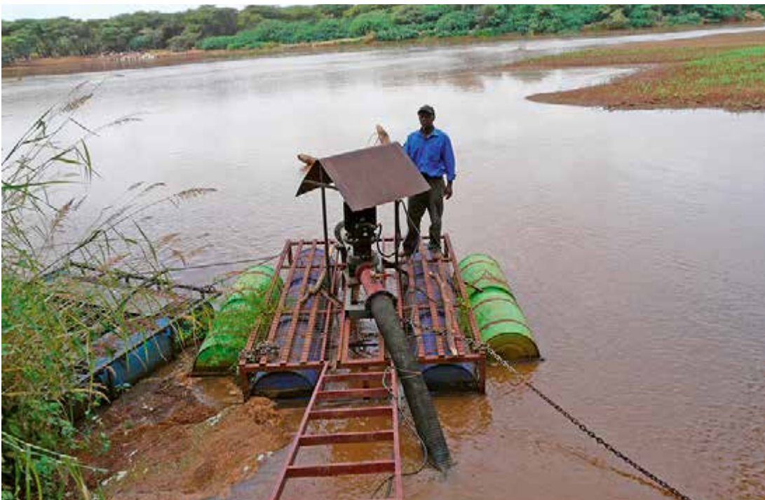
Figure 5.28: Floating solar water pump at Holgojo Farm, Kenya
