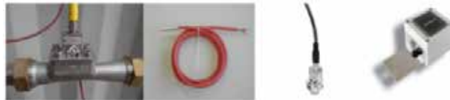
Figure 254: Flow-sensor, temperature sensor, pressure sensor and irradiation sensor (from left to right)
