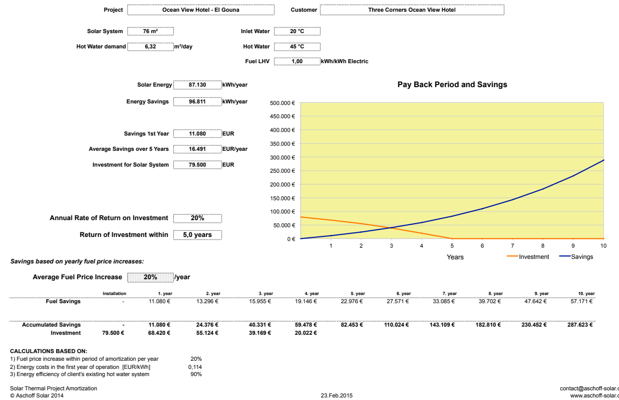
Figure 293: Amortization plan to replace the old solar thermal system of the 79-room building.
