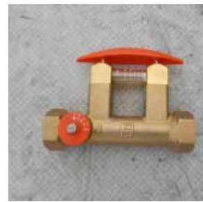
Figure 256: Balancing valve to have the same flow rate in each collector line and as the same temperature outlet of the collector field
