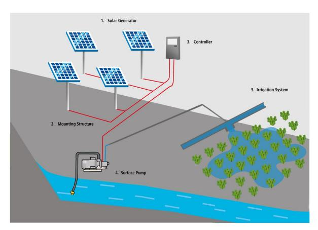
Simple configuration – with a tracking system – of the different components of an SPIS (Source: GFA)
