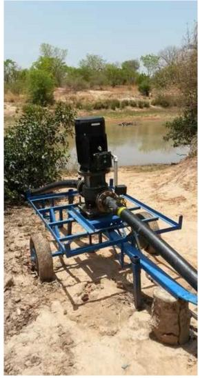
Surface pump on a mobile structure (Source: Lennart Woltering)
