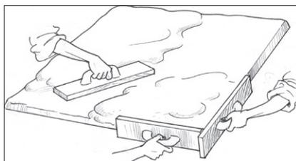
**1.4** Make the foundation slab as smooth and level as possible.
