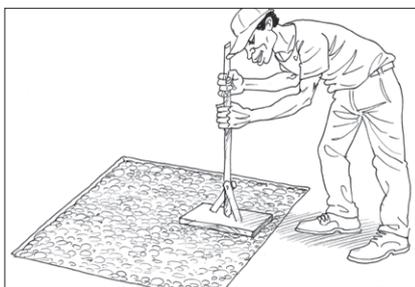
**1.3** Lay 6cm as your base using the mixture of clay with chopped grass or sawdust.
