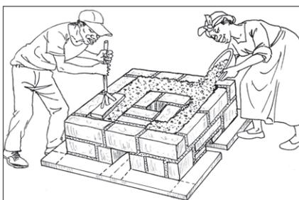
**4.1** Build up the second course of bricks for the outer wall, and mortar them into position. Make sure to check horizontal levels and height at all times.
