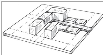
**2.5** Complete the roof of the air inlet with another layer of bricks. Mortar the bricks into position.
