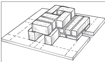
**3.2** Place the bricks for the outer wall of the stove, leaving space for insulation between the outer and inner walls. Mortar the bricks into position to complete the first course.
