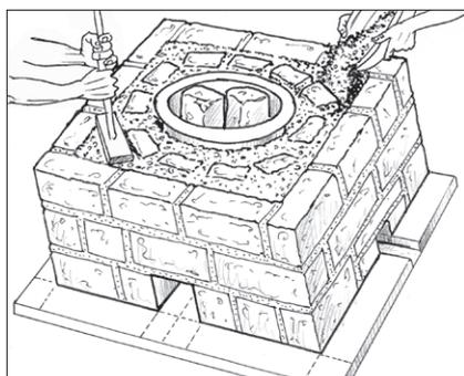
**6.4** Pour the clay mixture on the surface and spread out evenly. Smooth it to about 2.5 cm from the edge of the pot. Ensure that the stove's top surface is uniformly horizontal.
