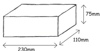
The rocket stove must be built using fired clay bricks of standard size, because then it is easy to observe proper dimensions for the stove, in particular the combustion chamber, during construction.
