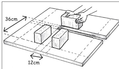
**2.3** Complete the left wall of the combustion chamber and use the clay mixture to fix the bricks into position.
