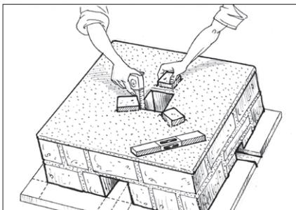
**5.1** Around the combustion chamber, place 3 pieces of cut brick to make the pot rests — 1 at the back wall, the other 2 on either corner of the front of the chamber. Add mortar as a base to hold the pot rests in position.
