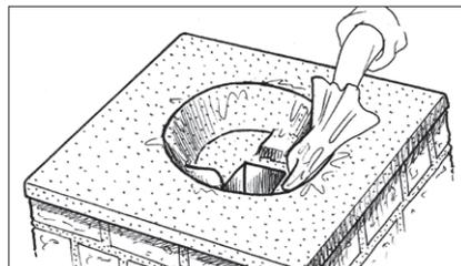
**7.5** Use the extra clay mixture to smoothen the sides and add finishing touches, such as the skirting around the stove. Leave the stove to dry for 3 weeks while covered with a watertight material e.g. polythene bag.
