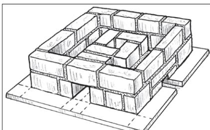
**4.2** Pour the clay mixture into the gaps between the combustion chamber and the outer wall, up to the level of the bricks. This is for insulation. Press down lightly to compact the material so little air remains.
