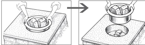
**7.2** On the surface of the mortar, draw a faint line all around the pot, using the outer brim of the pot as your guide.
