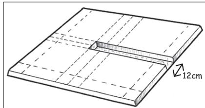
**2.2** Place 2 bricks in the front to mark the door of the firewood entrance. Place 1 brick on the back wall of the combustion chamber. The distance from the front to back should be 36cm.
