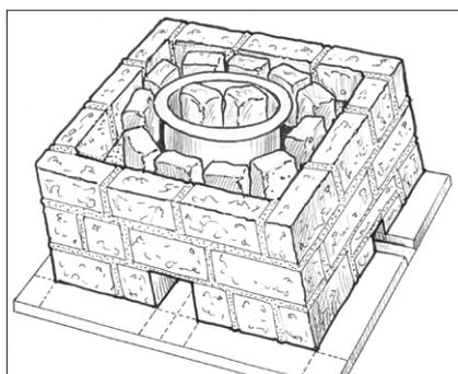
**6.3** Pour the clay mixture into the gaps between the pot and outer wall. Compact the insulating material, then sprinkle with little water as before to make the surface smooth.
