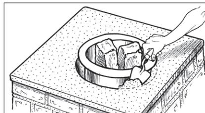
**7.4** Remove the pot and smoothen the sides of the pot rest area, using a little mortar. Wear a rubber glove or protect your hand with a plastic bag. Keep excess clay mixture for the finishing touches.
