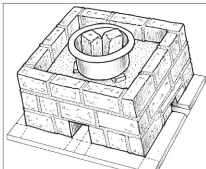
**6.2** Cut 4 or 5 bricks into half and stand the pieces in a circular pattern around the pot, making sure the pot is in the centre.
