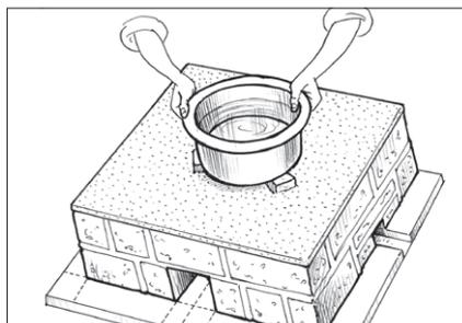
**5.2** Take the largest pot commonly used by the household, and place it on the pot rests. Check that the pot is level by filling it with water and seeing to the equal distribution of water in the pot. Adjust the mortar under the pot rests if necessary.
