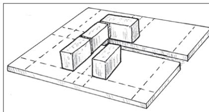
**2.4** Place 4 bricks on either side to line the length of the air inlet.
