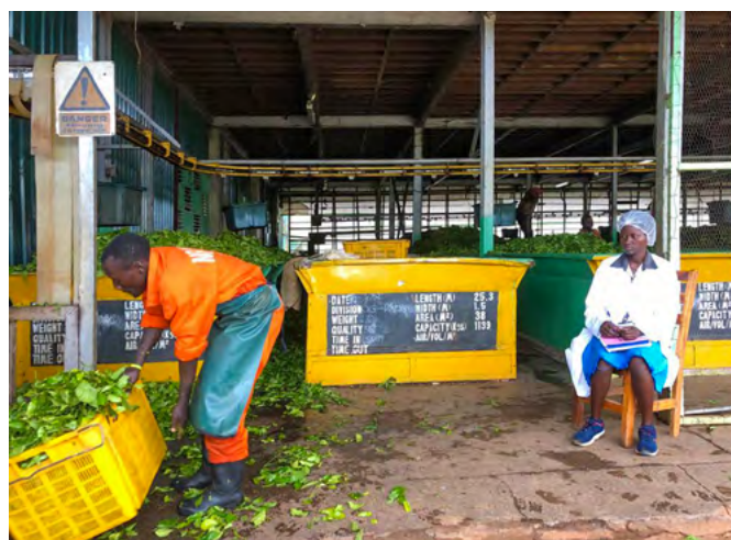
Figure 3: Tea withering process
