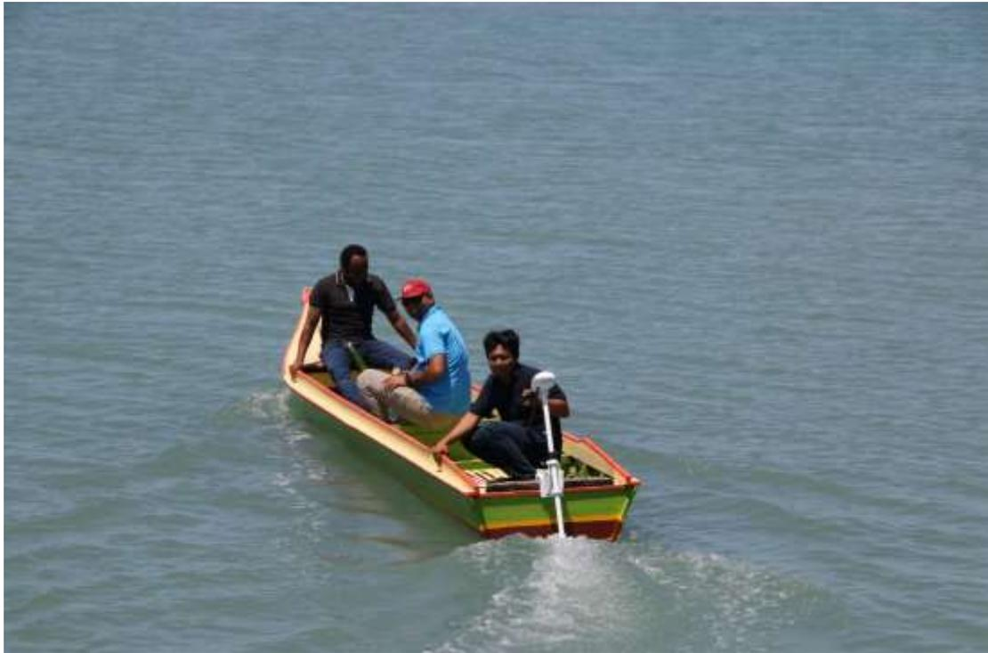
*Figure 9 Site visit to Sabangko Island. Participants tried the e-mobility solution renewable energy boat. The boat is powered by electrical outboard motors with battery charged by the PV system.*
