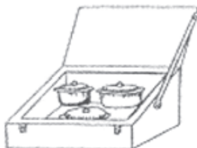
Fig. 5.g: Pots of food cooking inside an indirect solar cooker
