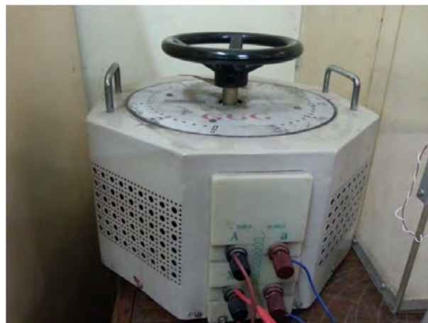
Fig. 3.3 Variac used for varying the power input
