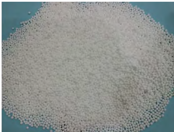
Fig.2.4 Polystyrene micro beads used as insulating material in WonderBag
