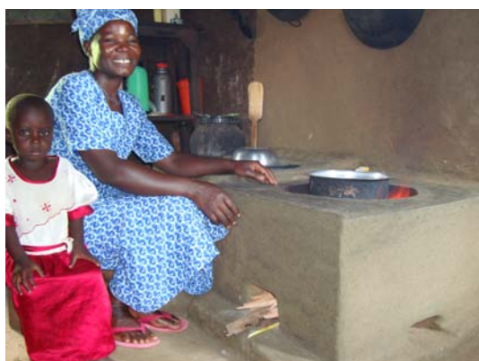
Rocket stove with two potholes
