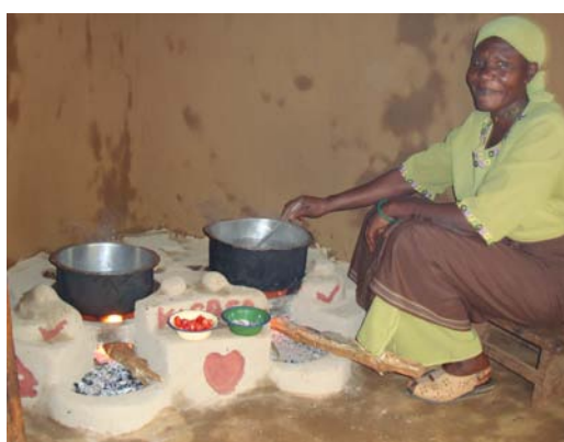
Jiko Kisasa with two potholes
