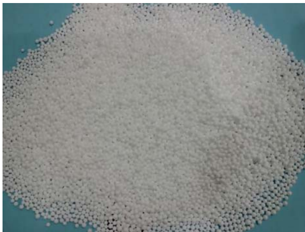
Fig.2.4 Polystyrene micro beads used as insulating material in Hot Bag
