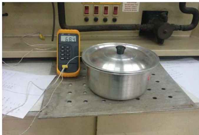
Fig. 6.5 Heat retention test without Hot Bag
