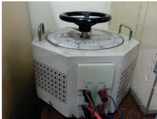
Fig. 3.3 Variac used for varying the power input
