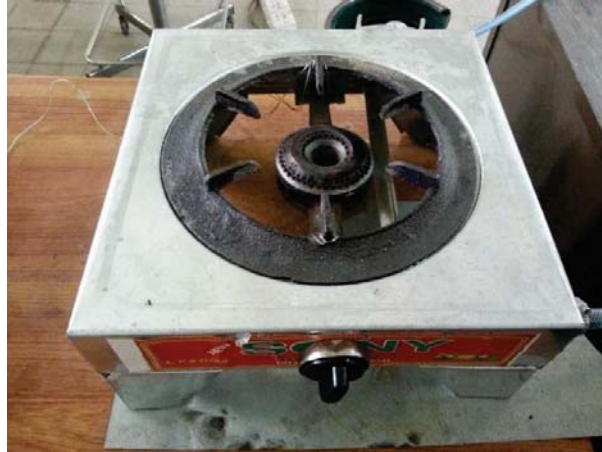
Fig.3.2 Single burner stove having LPG as fuel
