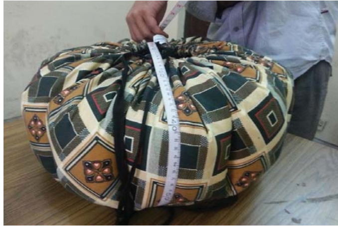
Fig. 6.13 Measurement of peripheral length vertically
