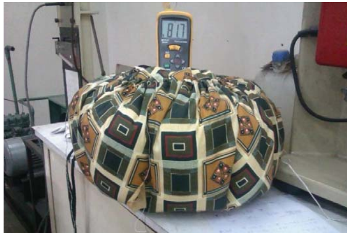
Fig. 6.6 Heat retention test using Hot Bag
