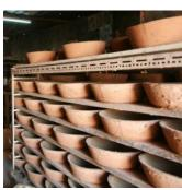
After drying, the liner is fired in a pottery kiln and delivered to the local tinsmiths who then assemble the final product:
