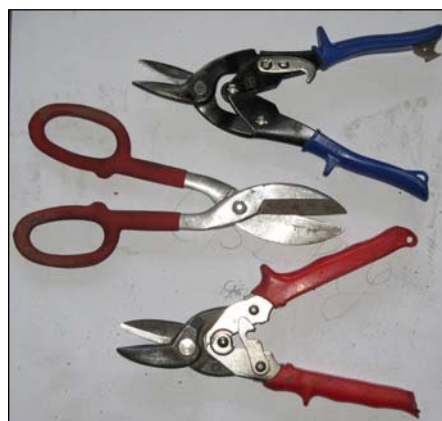
Of the hand scissors pictured above, only the one with the blue handles was of good quality to cut thin 0.4 mm to 0.7mm GI sheet.
