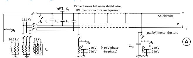
Figure A5.8. Single Line Diagrams of "Single-phase Ground-return" SWS
