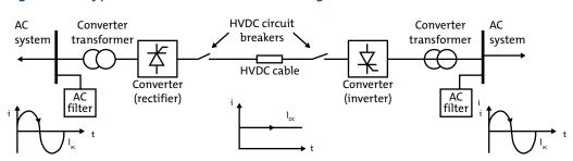
Figure A5.5. Typical HVDC Interconnection Arrangements
