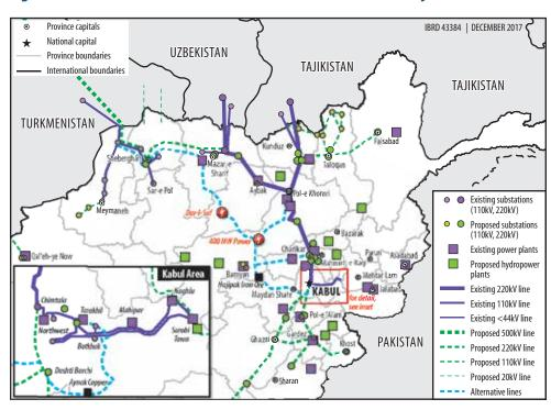
Figure A5.4. Alternative Transmission Routes to Provide Diversity in NEPS
