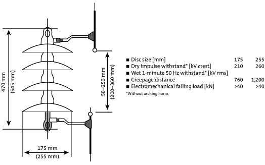
Figure A5.9. A Rigid String Toughened Glass Insulator String with Arcing Horns, As Used in Northern Ghana
