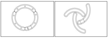
Figure 4: 3 sections gounziye in full circle and in configuration for pots and pans
