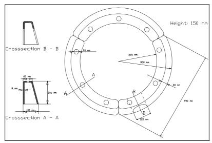
Figure 10: Design drawing aluminium gounziye
