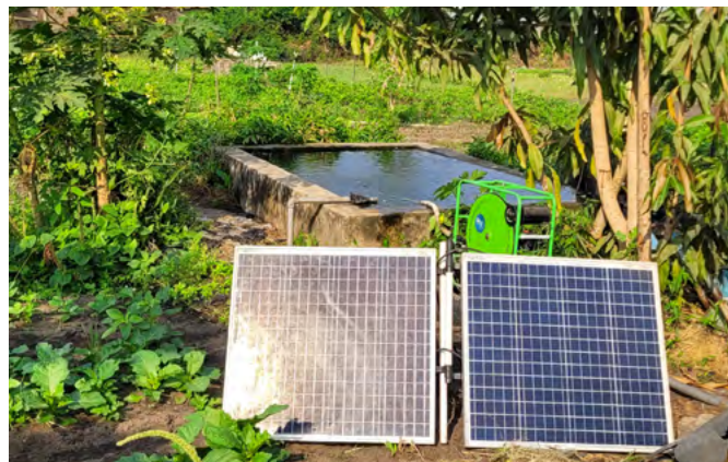
Picture 2: Mobile solar pump
