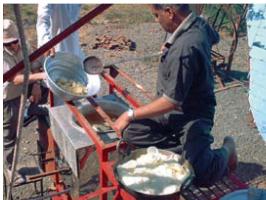
Photo: Deepak Ghadia-Frying potato crisps with an 8 sqm Scheffler-cooker
