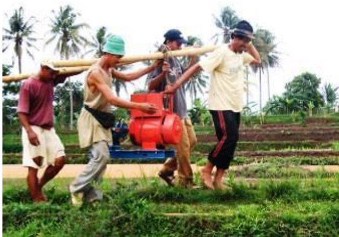
Figure 8 Transporting a turbine across a paddy field
