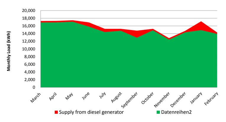
Energy share curve of a 200kWp Solar-Diesel Hybrid Minigrid Renewable Fraction > 90%
